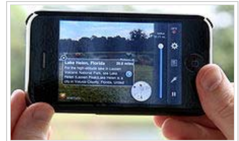
Wikitude World Browser on the iPhone 3GS uses GPS and a solid state compass
