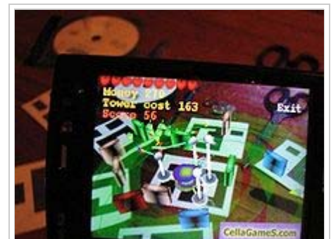
AR Tower Defense game on the Nokia N95 smartphone (Symbian OS) uses fiduciary markers
