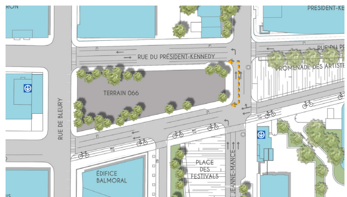
Figure 9 : incorporation of the west side traffic lane of Rue Jeanne-Mance
