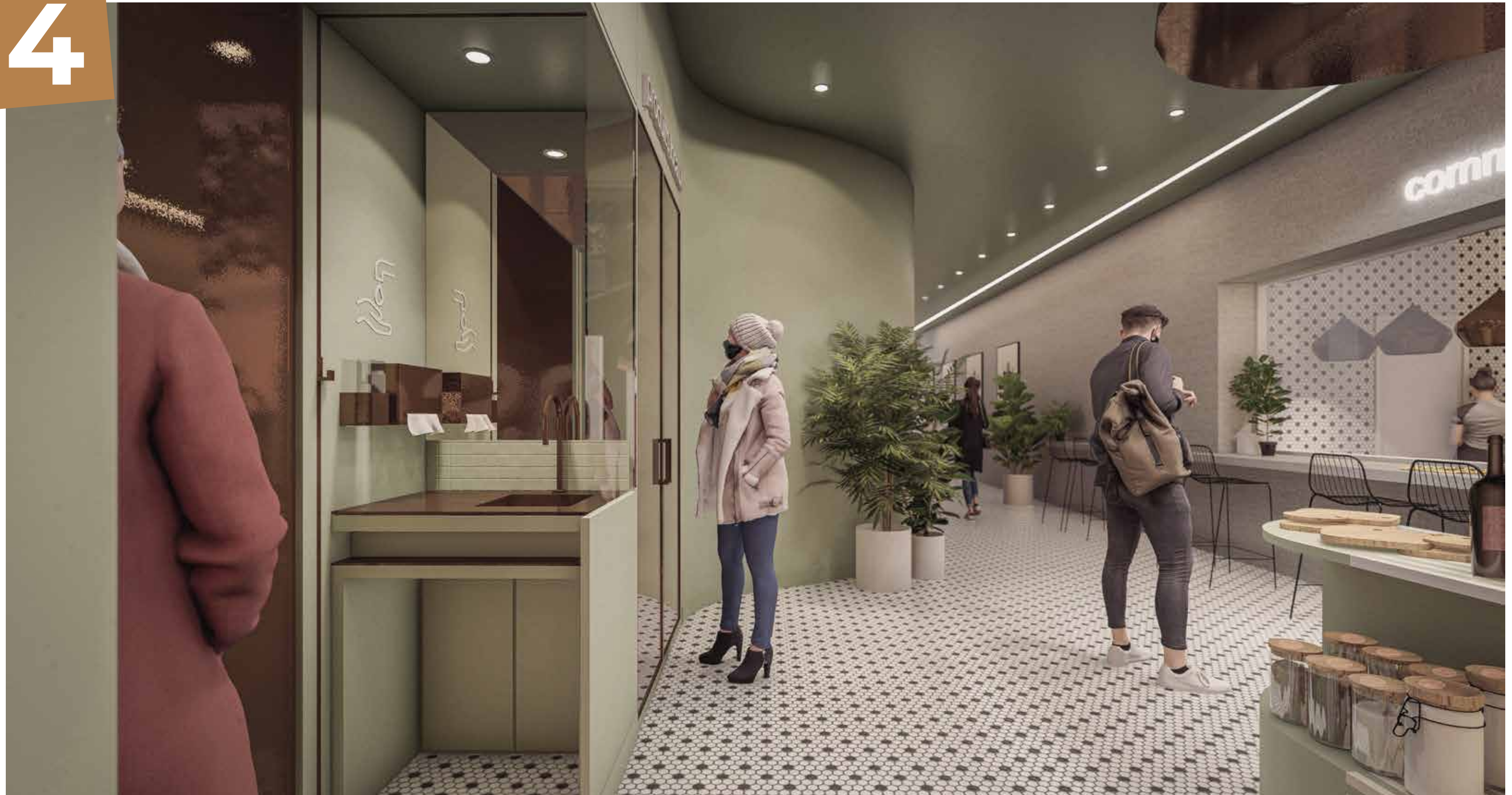
Contactless, universally accessible handwashing station • Functional elements: hook, hand dryer, etc. • Unobstructed traffic area • Components visible to staff • Easy-to-clean materials • Products showcased
